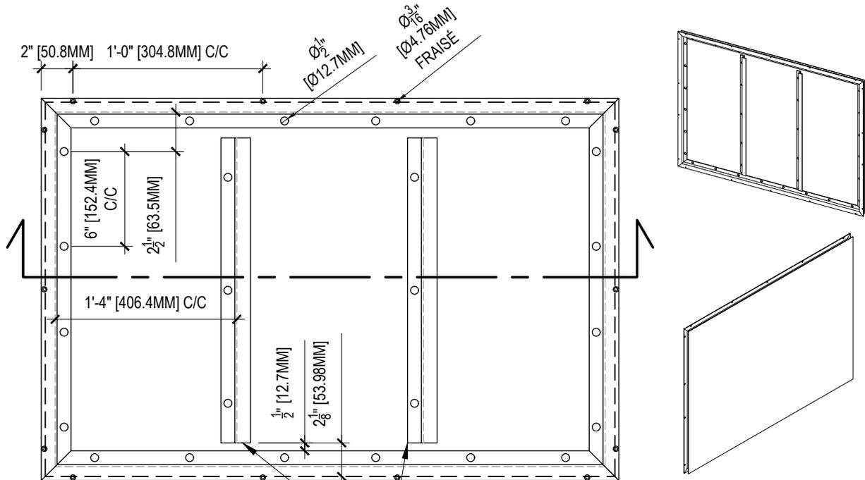
RENFORTS EN ALUMINIUM EXTRUDÉ EN "Z", DE 1/8" [3.2MM], POUR LES PANNEAUX AUX DIMENSIONS SUPÉRIEURES À 2'-0" x 2'-0" [609.6MM X 609.6MM].
